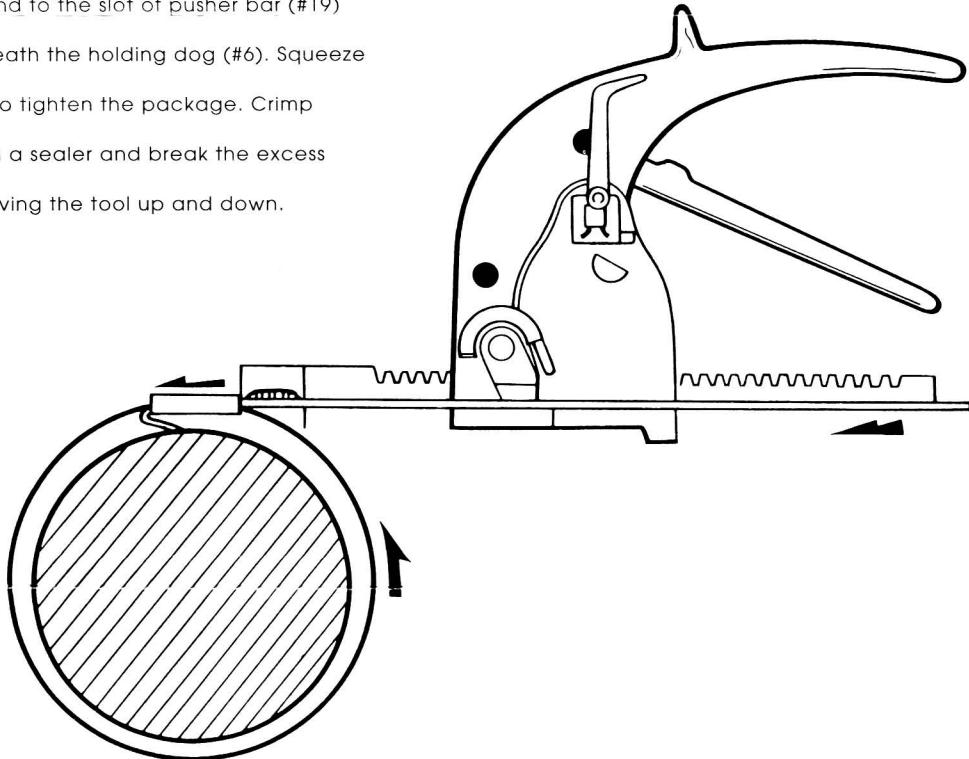
Keep the tool well oiled, and the screws and bolts tight.
