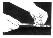
Slide the strap through the seal. Note position of seal, with lugs held up and away from the operator.
