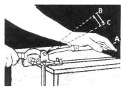
9. If strap needs further tightening, pull long handle back from position "A" to position "B". Tighten strap with short easy strokes from "B" to "C".
