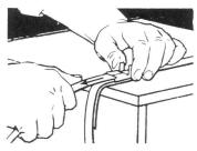
Pull strap tightly around box and through seal. Note 1inch distance between seal and box edge, also correct position of underflap.
